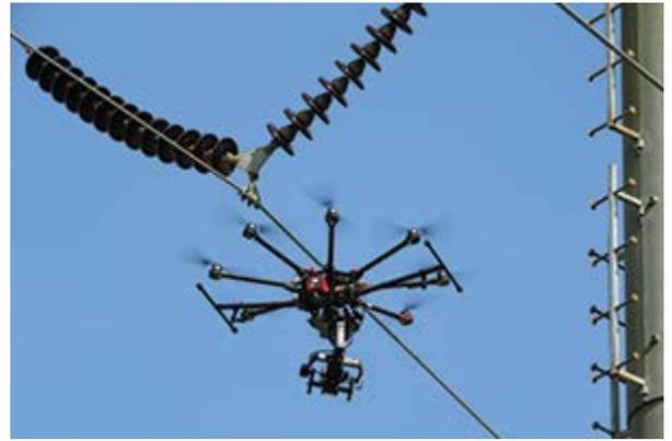
Dominion is using drones to inspect transmission lines and structures ranging from wooden utility poles to transmission towers that are 200 or even 500 feet high. Drones allow Dominion to make inspections from more angles than it could achieve with a helicopter. Using drones for inspections, however, costs about the same as using helicopters, according to Steve Eisenrauch, manager of electric transmission forestry and line services for Dominion Virginia Power.
